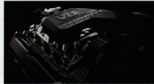
Town Car's 210-horsepower V-8 engine employs overhead cam design and a unique roller rocker arm valve train for low internal friction and excellent operating efficiency.
