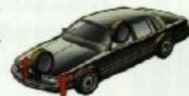
The short and long-arm (SLA) independent front suspension is designed to counteract "dive" when braking.
