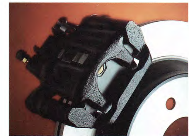
The 11.65-inch rear brakes are clamped by single-piston calipers. The rotors feature internal cooling vanes.
