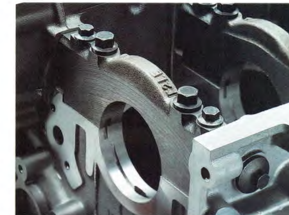
The nodular iron main bearing caps attach to the block with not two or four, but six bolts, spreading tension and load over a greater area of the block, endowing the bottom end with tremendous strength.
