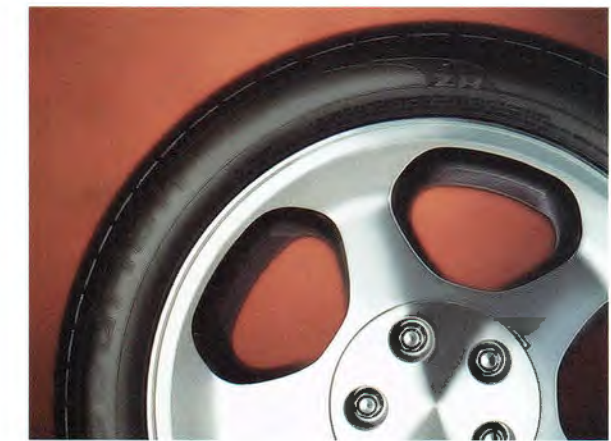
The Cobra's 17.0-inch five-spoke alloy wheels are wrapped with BFGoodrich Comp T/A ZR radials, which are derived from the Comp T/As fitted to SVT's 1995 Mustang Cobra R race car.
