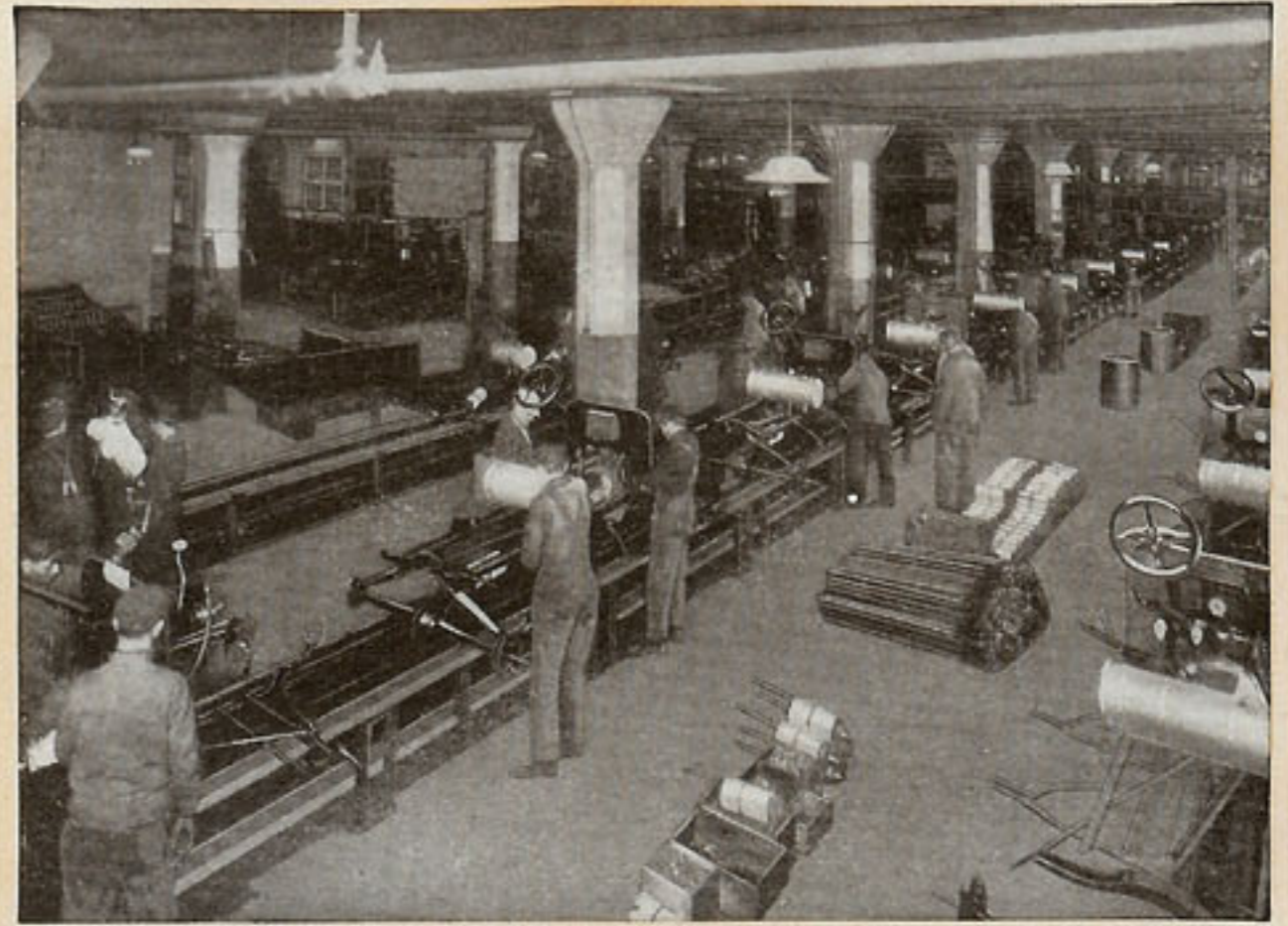
On this traveling assembly line, moving 8 feet per minute, the Ford chassis grows, unit by unit, into a completed motor car
