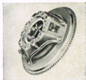
Heavy-duty 11" clutch is the positive-action type. (Standard on "Interceptor" V-8 with Conventional Drive or Overdrive.)
