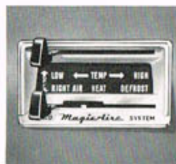
Comfortable temperatures are maintained by Magic-Aire Heating-Ventilating System (controls shown), or by the recirculating type heater-defroster.
