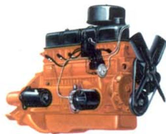
New 139-hp 223 Six—the only modern Short Stroke Six in Light and Medium Duty trucks today!
