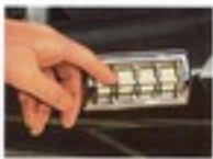
Lincoln Power Windows glide up and down at the touch of a button. There's a separate switch at each window, and driver has a master window control. Naturally adjusted to operate only with engine running.
