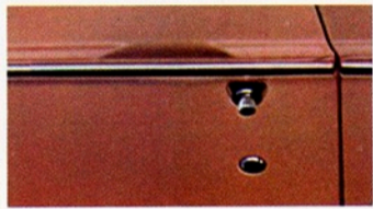
New Flow-Line door handles blend into the body side molding. Hand-hold recess areas are sculptured into the doors behind the handles.
