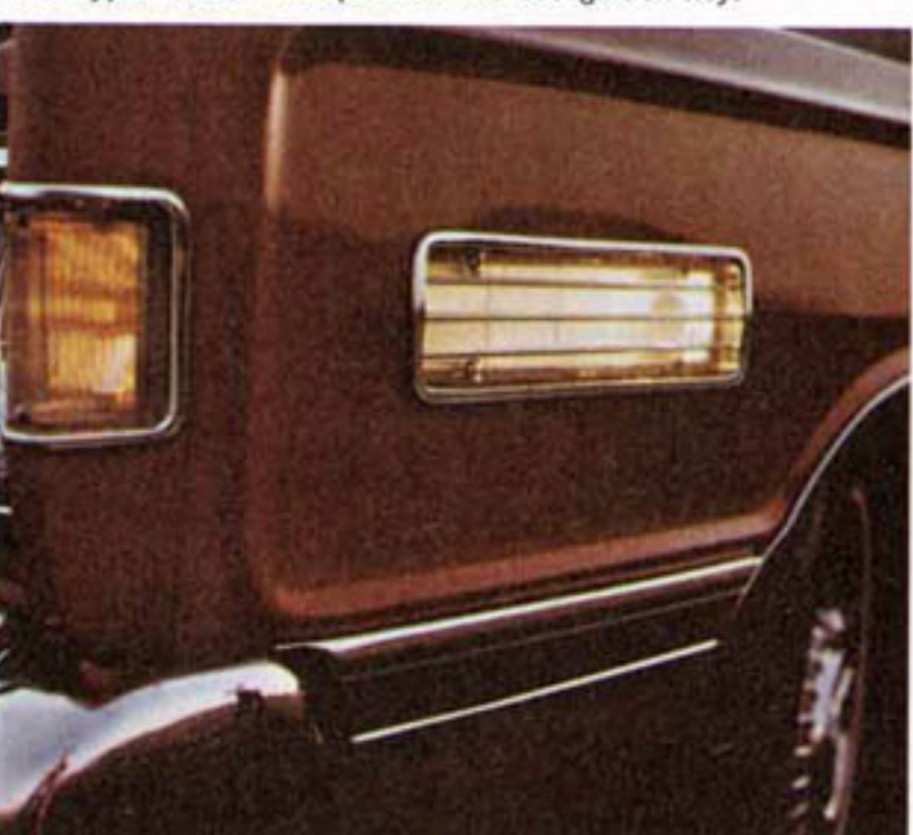
CORNERING LIGHTS throw a floodlight beam through 120° arc from direction of car. Actuated by turn signal.
