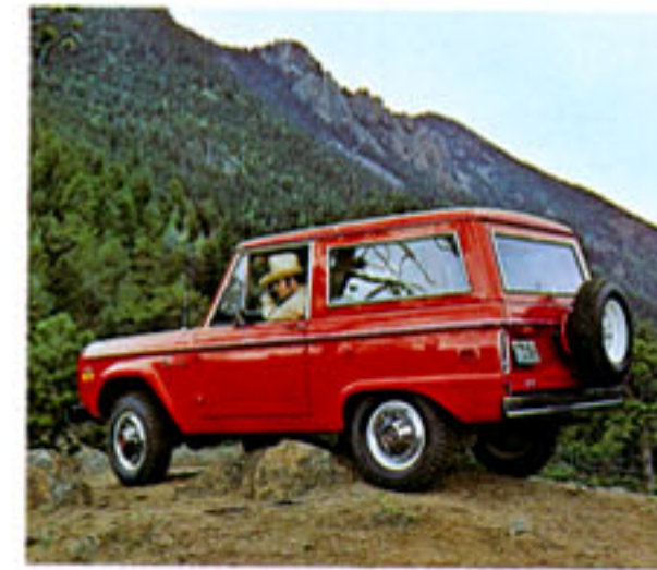
Excellent ground clearance. Bronco combines the best ground clearance amidships (w/optional 6.50 x 16 tires) with a big ramp breakover angle to allow crossing over high projections. Bronco's excellent angles of approach and departure provide greater freedom from hangups when approaching or leaving steep inclines and ditches.
