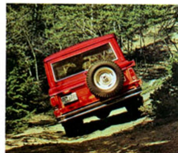
Slope-hugging stability. Bronco has the optimum track width. Wheels are set wide apart for excellent off-road stability, yet narrow enough to negotiate twisting paths and trails. And Bronco's "identical track" front and rear axles allow the rear wheels to follow in the same path made by the front wheels for easier trailblazing.
