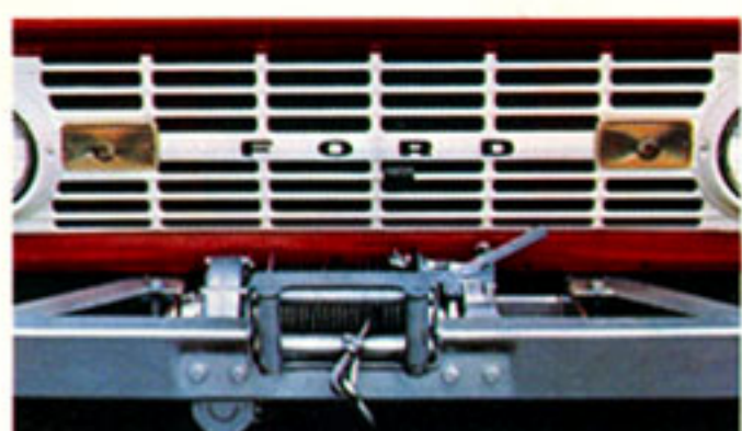
Front-Mounted Winch with 150 feet of 5/16-in. cable is power take-off driven.
