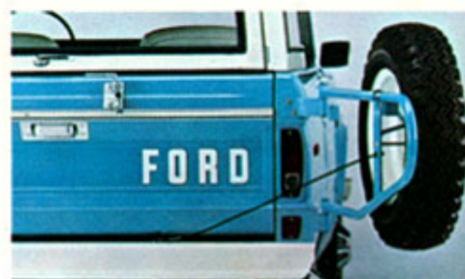
Swing-Away Spare Tire Carrier puts spare out of the way for more cargo or luggage area, easier access.
