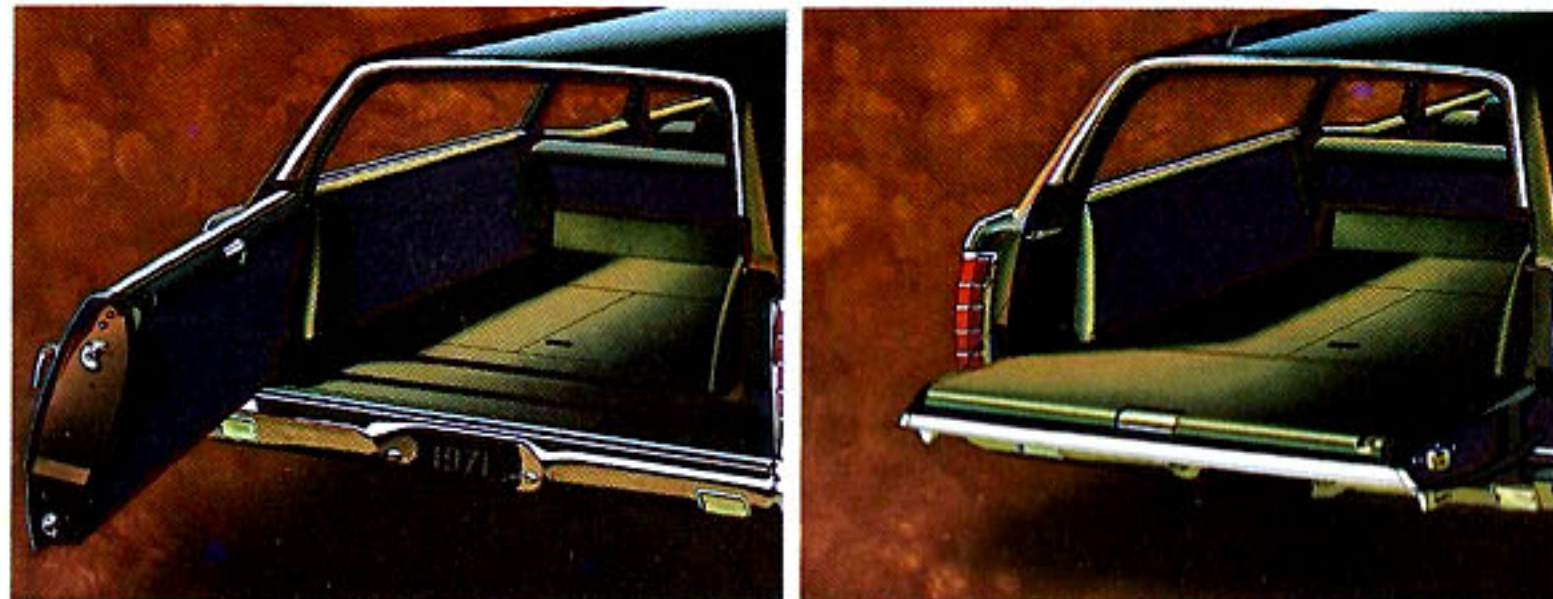
Dual-Action tailgate: swings wide like a door for passengers, down like a tailgate for cargo!
