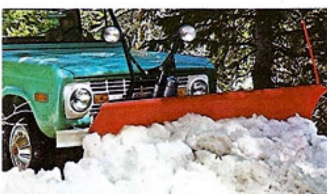
Snowplow Blade may be adjusted easily to various heights and angles (with kit) from within the cab.
