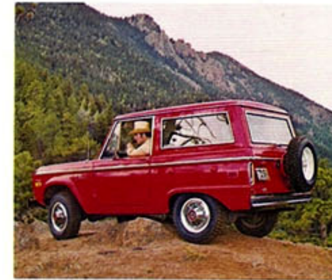
Excellent ground clearance. Bronco combines optimum ground clearance amidships with a big ramp breakover angle to allow crossing over high projections. Bronco's excellent angles of approach and departure provide greater freedom from hangups when approaching or leaving steep inclines and ditches.
