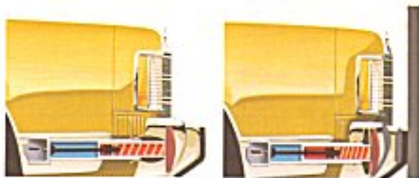
Hydraulic bumper system absorbs minor impact.
