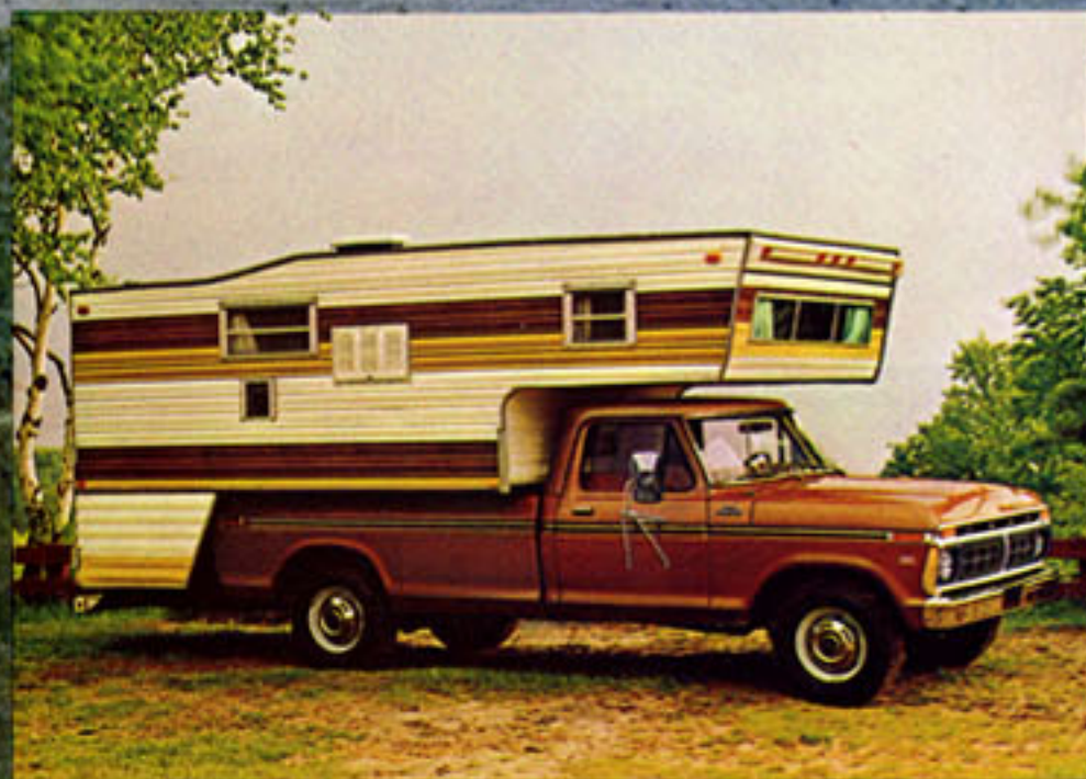
Regular Cab Campers. Regular Cab Pickups accommodate up to 12-ft. slide-in campers. Chassis-Cab models take up to 14-ft. campers. Ranger shown with camper package.
