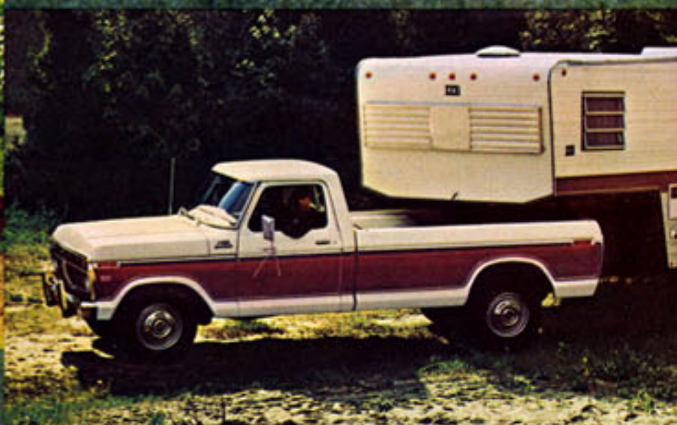
Trailer Towing Packages. Ford offers optional Light and Heavy Duty packages to match your hauling needs. Gross Combination Weight Ratings up to 15,000 lb. for 5th wheel trailers and 18,500 lb. for conventional trailers. Ranger shown with deluxe Tu-Tone, protection package and radio.
