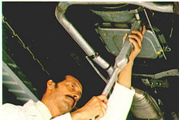
Underbody bolt torque inspection
