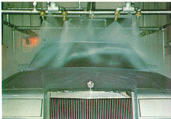
High pressure water leak test
