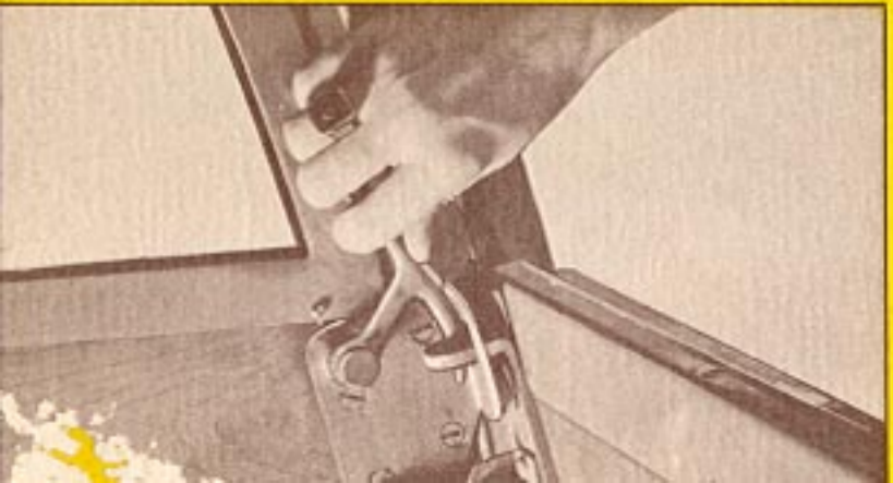
This ingenious fastening assures a securely locked tail-gate and eliminates rattles at that point. The tail-gate can be fastened either from inside or from outside the car. Window above tail-gate is easily opened.
