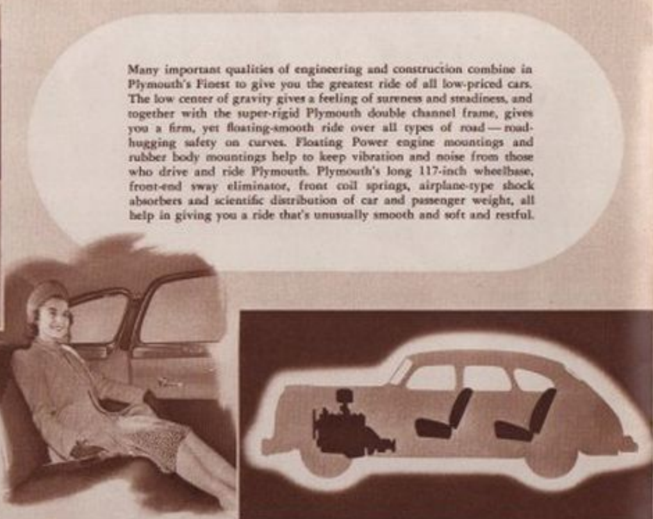
Rubber-poise Body Mountings are designed to eliminate metal-to-metal contact between body and frame, and to absorb road noises and vibrations.
