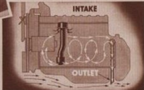
Complete crankcase ventilation contributes greatly to long life by carrying off the injurious vapors that form in crankcases, to prevent dilution of oil and to protect important engine parts against corrosive action.
