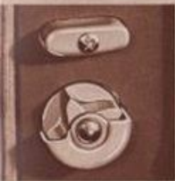
Rotary-type door latches have a continuous "take-up" to tighten doors as you ride along — safety!
