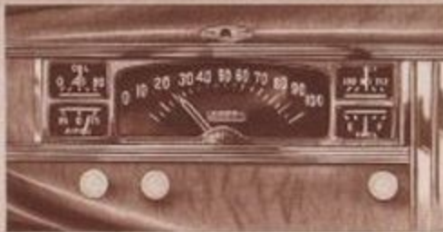
Plymouth's Safety Signal Speedometer changes color to warn of speed changes. When lighted, the dial is green up to 30 miles per hour, amber from 30 to 50 and red above 50. This enables the driver to know at a glance if he is driving at a dangerous speed.
