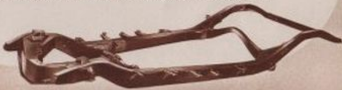
Plymouth's super-rigid, double channel frame supplies great steadiness to the body, and by lowering the center of gravity, contributes to safety on curves. It furnishes a solid foundation for the famous Plymouth Safety Steel Body. Safety, long life.
