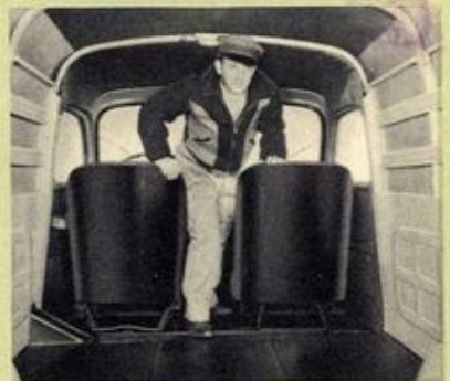
Where tilt-back auxiliary seat is used, there is plenty of room between the two seats for a driver or helper to slip easily into the rear compartment.
