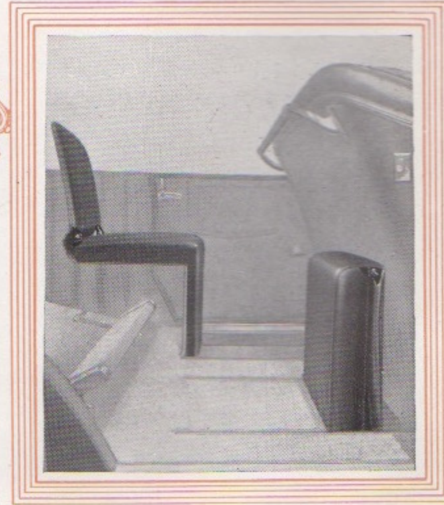
These views show the auxiliary seats ready for use and when folded away. Note the design, also how neatly the seats fold up.
