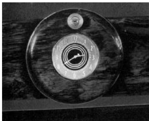
• ELECTRIC PANEL CLOCK —Designed for door of package compartment and styled to match the instrument dials. Indirectly illuminated for night driving.
