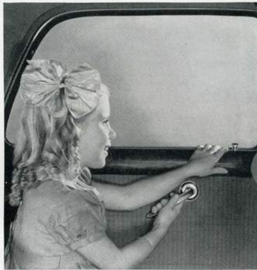
Safety Catches on rear doors prevent doors from opening accidentally while car is in motion.
