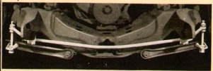
FRONT AND REAR RIDE STABILIZERS. Control rolling motion and prevent body sway on turns and curves. The results are greater driving ease, riding comfort and safety.
