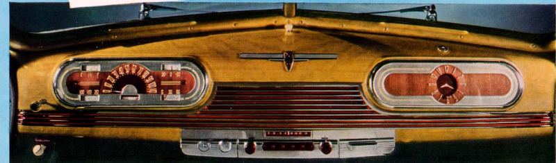
De Luxe Instrument Panel. All de luxe models in Series 66, 68, 76 and 78 have de luxe instrument cluster with clear vision plastic facing, de luxe clock and glove compartment door, and automatic glove box light.
