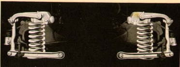
DOUBLE-ACTION HYDRAULIC SHOCK ABSORBERS. Proved cam and lever design. They control vertical motion, absorb road shocks, and take up rebound.
