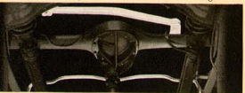
↑ LATERAL STABILIZER BAR. One end anchored to frame and the other to rear axle. Prevents side-to-side movement and keeps frame and rear axle in alignment.
