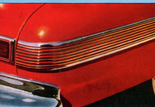
Chromium Trim on Rear Fenders. Series 76 and 78 de luxe models have chrome speed lines on rear fenders. Not included on models of Series 66 and 68.
