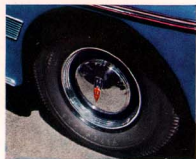
7.00 x 15 inch tires with 5.50 inch rims give better traction and longer wear.
