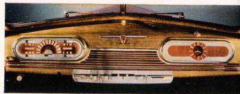
De Luxe Instrument Panel in Series 66 and 68. Instruments are grouped directly in front of the driver. A light in the glove compartment flashes on automatically when door is opened.
