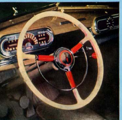
All de luxe models have cream colored plastic steering wheels with ring-type horn control.
