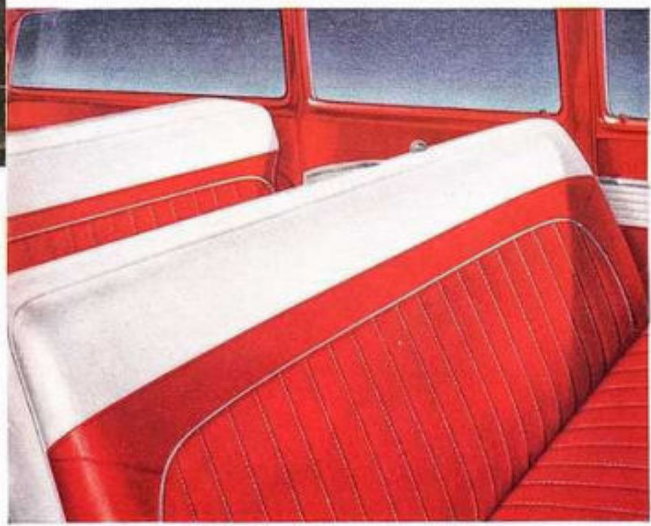
IN THE CHIEFTAIN FOUR-DOOR SAFARI as shown—the second seat folds for access to the rear seat . . . rear seat is removable, providing a floor length of over 4 feet. With rear seat removed and second seat folded flush with the floor, floor length is jumped to nearly 7½ feet.
