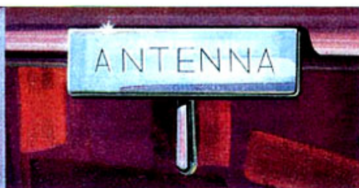
BUICK ELECTRIC RADIO ANTENNA —Controlled by lever under instrument panel on driver's side—raises and lowers antenna while driving or while stopped.
