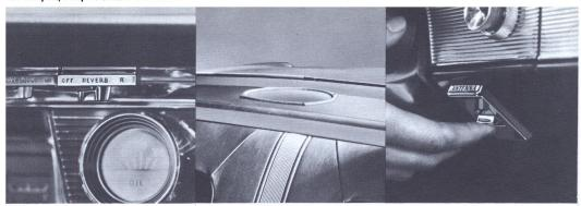
Verbra-Phonic Rear Speaker System—New dimension in sound. Fraction of second delay of sound from rear seat speaker simulates concert hall acoustics. 3-step instrument panel switch allows selection of front or rear speaker, or both.
