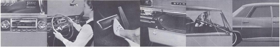
Tri-Comfort Circ-L-Aire Conditioner-All new system supplies dehumidified heated or cooled air to desired temperature-reduces dust and pollen in car. Control unit for Catalina, Star Chief, Bonneville, and Grand Prix illustrated.
