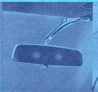
Non-Glare Inside Rear-View Mirror— Center finger tab on bottom edge permits easy snap adjustment for safer non-glare or nighttime driving. Reduces eyestrain and fatigue.
