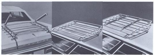
Rear Deck Ski and Luggage Carrier—Convenient rear deck location makes loading easier—use for skis only or convert to full load capacity—store when not in use. All models except Safaris.
