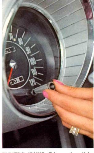
ELECTRO-CRUISE—Take your foot off the accelerator — speed is maintained automatically. Optional on LeSabre, Wildcat, Electra 225, and Riviera only.
