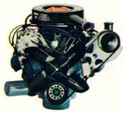
WILDCAT 355-300 cubic inches of get up and go that puts out 250 h.p. This 4-barrel carburetor V8 is available on Special, Special Deluxe, Skylark, Sport-wagons and Le Sabre. Goes with Super Turbine (optional) or with the regular 3-speed synchromesh or 4-speed synchromesh (optional) transmissions (except
