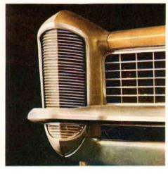
Something new in Riviera headlights. They're moved from the grille to a position behind the shields in the fenders. How do you open the shields? Simple, just pull the switch, they pop up out of the way. Push it in and the shields go down. Good way to amuse your friends.
