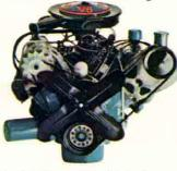
FIREBALL V6-a 225 cubic inch engine that turns up 155 h.p. Smart performance. Great regular gas economy. Available on Special, Special Deluxe and Skylark. Team it with Super Turbine (optional), regular 3-speed synchromesh or 4-speed synchromesh transmission (optional)
