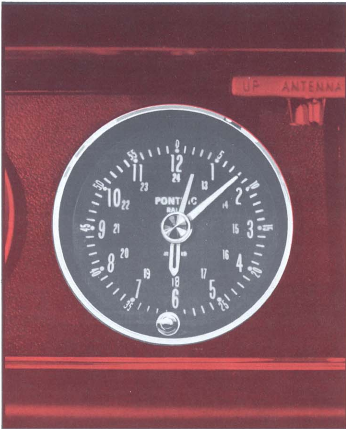
Tempest Rally Clock (Code 604) . . . smartly restyled, features sweep second hand, built-in self-regulator and illuminated dial. (Note: Not available with Rally Cluster option.) (F,D)
