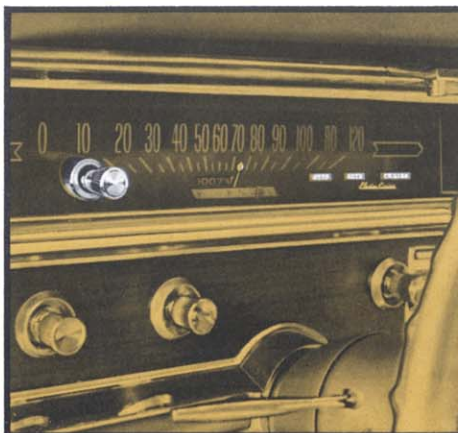
Electro-Cruise System (Code 514) . Automatically maintains driver-selected car speed. When automatic feature is not used, signals when pre-selected speed is reached or exceeded. Also gives low fuel warning. Available only with Turbo Hydra-Matic. (F,D)
