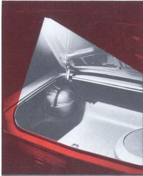
Luggage Lamp (Code 481) . . . automatically turns on when trunk is lifted (sedans and coupes only). Under-hood Lamp (Code 404) . . . automatically turns on when hood is opened. (D)
