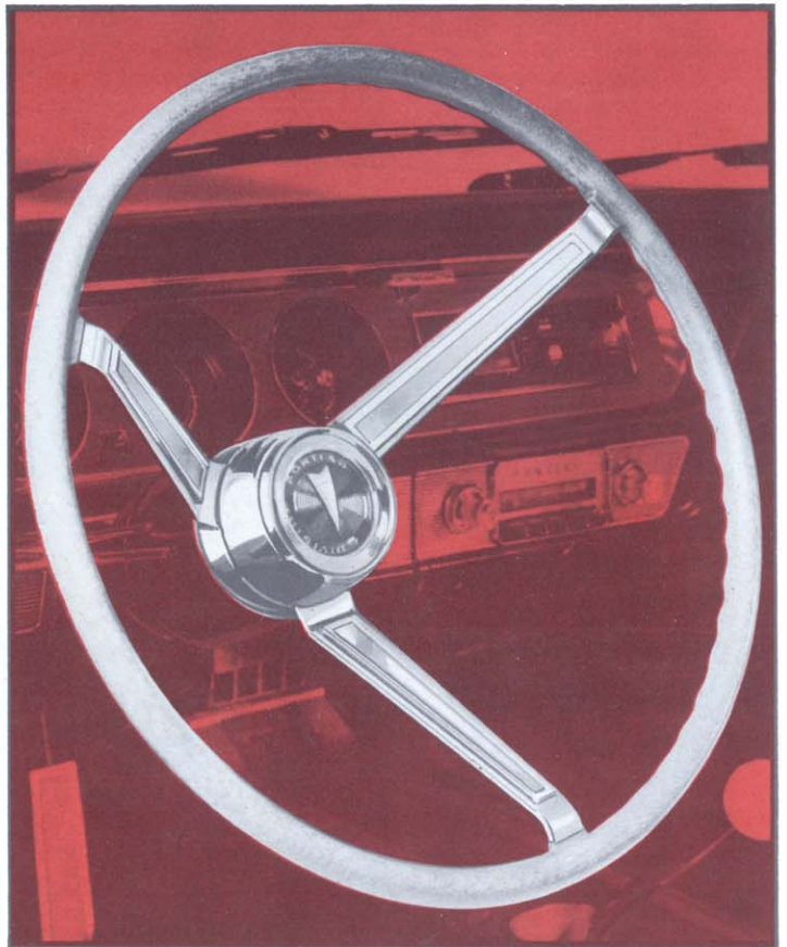
Custom Sports Steering Wheel (Code 524) . . . completely redesigned for 1965 to present a more symmetrical and pleasing appearance. Three equally spaced stainless steel spokes. Optionally available on all Tempest models, it can be ordered also when the tilt-wheel is selected. (F)
