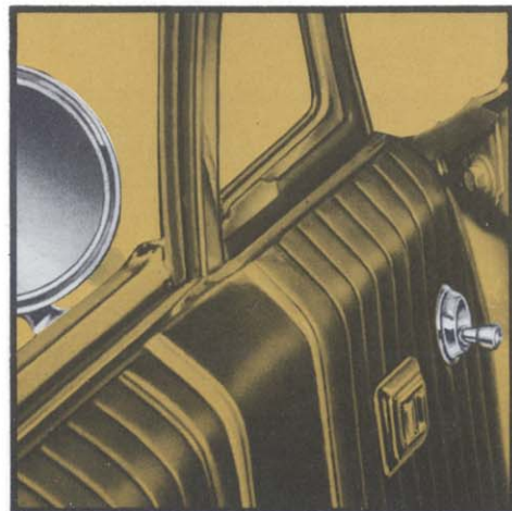
Remote-control Outside Mirror (Code 444) . . . restyled for 1965 and mounted on door to provide a greater field of vision—safer! Easily adjusted from inside car. Front surface chrome-plated to assure sharp, clear image and prevent blurring or ghosting. (F,D)
