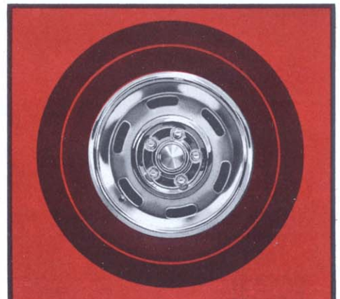
Rally Wheels (Code 691) . . . with special 7.75 x 14 tires only. Highly functional as well as extra sporty. Large openings provide maximum cooling for brakes. Includes stainless steel cap, chrome plated wheel nuts and stainless steel full trim ring. (F)
