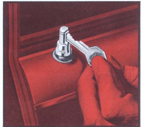
Rear Door Safety Locks (4-door models only) . . . prevent children from opening rear door. When lock button is pushed down, rear doors cannot be opened without inserting key in lock button. (D)
