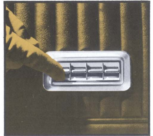
Power Window Lifts (Code 551) . . . automatically operate all vertically opening windows from a single control panel at the driver's side. Individual control buttons near each window. (F)
