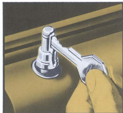
Rear Door Safety Lock (4-door models only) . . . prevents children from opening rear door. Once lock button is pushed down, rear doors cannot be opened without inserting a key into lock button. (D)
