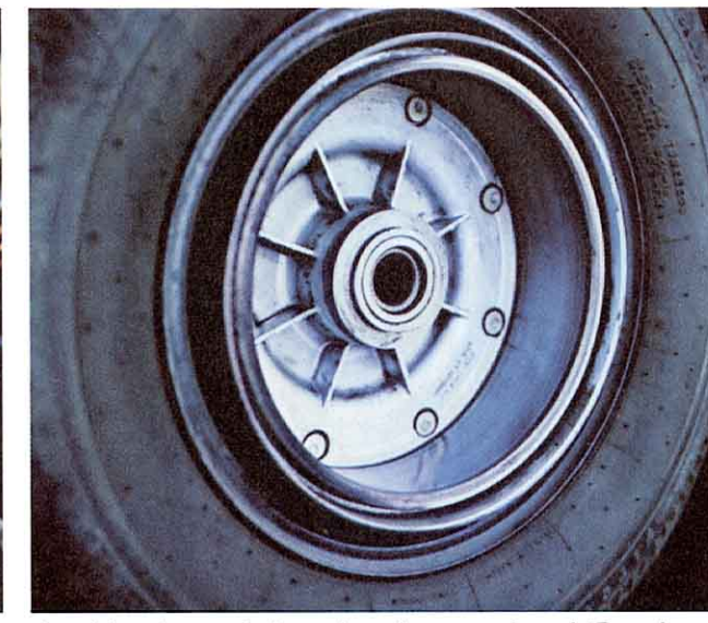
Inside view of the aluminum wheel. See how drum and wheel hub are cast together.
