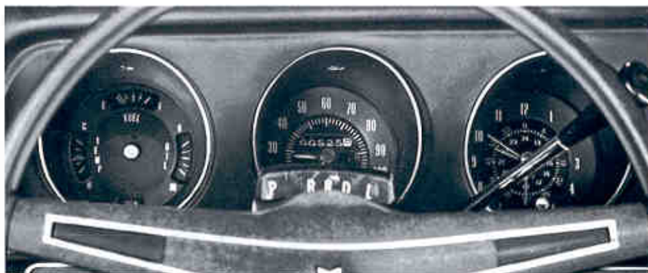
Rally Gauge Cluster & Rally Clock (Code 484—UPC W63). Integrates speedometer, oil-water-fuel-battery monitors and sweep second hand rally clock. Or rally clock can be replaced with Instrument Panel Tachometer
