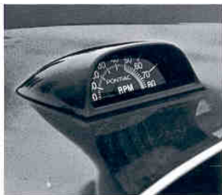
Hood-mounted Tachometer (Code 471—UPC UB5). Front-of-the-windshield installation lines it up for easy, instant readout by driver. Available Firebird, Tempest, Custom S, LeMans and GTO models. (F,D)
