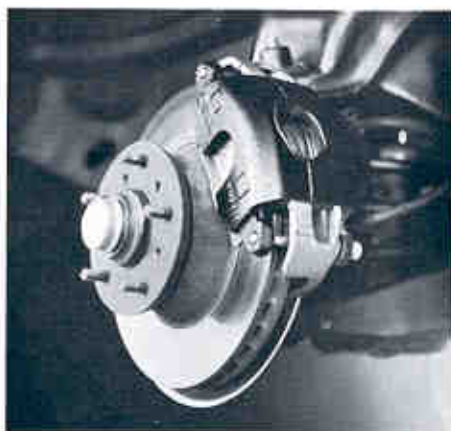
Power Disc Brakes, Front (Code 511—UPC JL2). New single-piston, floating-caliper design provides same braking area as 4-piston type. Power assist standard with disc brake. Available all models. (F)
