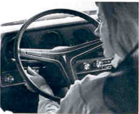
Tilt Steering Wheel (Code 504—UPC N33). Set at any one of seven different positions. Makes exit and entrance easier. Provides more lap room and can be changed from one position to another for more relaxed driving. (Available for all models with power steering. Not available with manual transmission, column shift.) (F)
