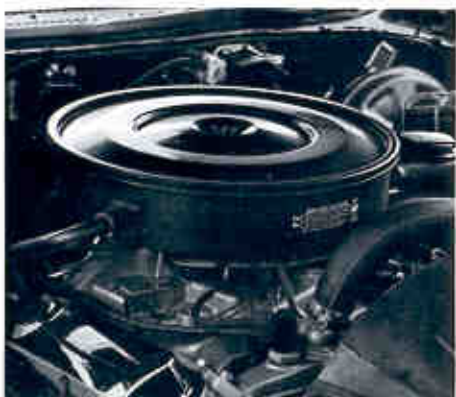
Dual-stage, Heavy-duty Air Cleaner (Code 731—UPC K45). Dual-filter design consists of wetted paper in filter, surrounded by polyglycol wetted polyurethane foam outer filter. Fine filtration, extended-surface. Available all models except those equipped with 428 H.O. engines. (F)
