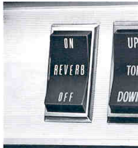
Verbra-Phonic (Reverberating) Rear Speaker System (Code 392—UPC U84). Available all models except Firebirds and those equipped with Stereo AM/FM Radios (Code 388), Stereo Tape Player (Code 394) or power ventilation (Code 588). When both front and rear speakers are playing, an "in-depth" tone is created that resembles the acoustics of a concert hall. (F,D)
