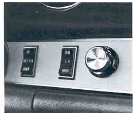
Power-flow Ventilation System (Code 588—UPC C57). Helps improve air circulation on models with upper-level ventilation system, especially while stopped at traffic lights. Features a blower fan ahead of each outlet (available all models with upper-level ventilation system). (F,D)
