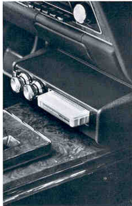
a control for balancing the volume between front and rear speakers. Plays the popular 8-track tape cartridges. Available only with radio. (Not available on Grand Prix or cars not equipped with heater.) (F,D)
