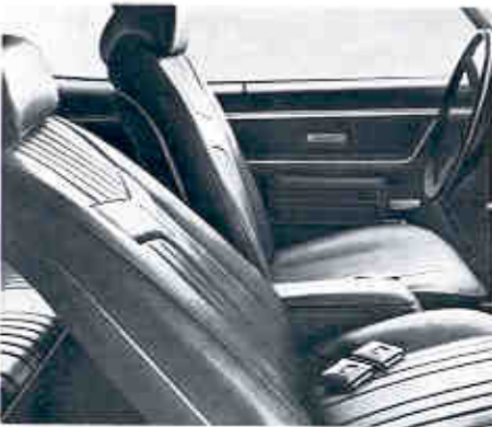
Reclining Bucket Seat, Passenger Side (Code 578—UPC A70). Available LeMans, GTO, Catalina, Bonneville and Grand Prix models with Strato-bucket seats. Passenger side reclines to 45° angle. (F)
