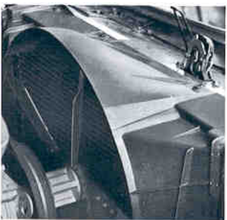
Heavy-duty Radiator (Code 701—UPC V01). Has greater cooling capacity, standard with air-conditioned cars. Available for all models. Also, SUPER-COOLING, HEAVY-DUTY RADIATOR (Code 702—UPC V02), for cooling under most severe driving conditions. Available for Catalina, Executive and Bonneville. (F)
