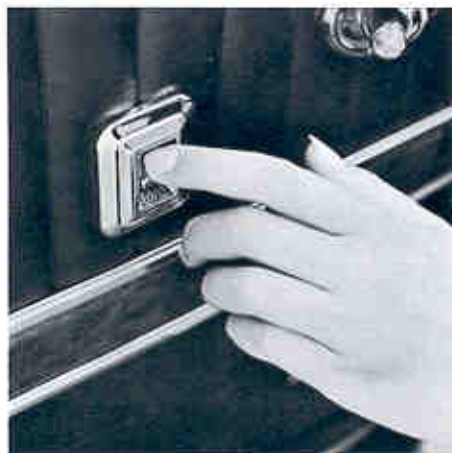
Power Door Lock System (Code 541—UPC A93). All doors are locked or unlocked at the same time by a master control lever on the
