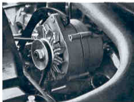
Delcotron Alternator-Regulator (62-Amp. Code 681—UPC K81; 55-Amp. Code 682—UPC K82; Self-regulated 55-Amp. Code 688—UPC K96). Special "solid-state" voltage regulator, built into the alternator, provides improved voltage control and added reliability—increases battery life. Available for all series equipped with V-8 engines. Style and amperage determined by engine or equipment. (F)
