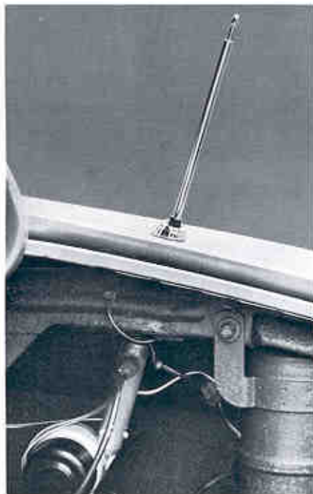
Electric Power Antenna (Code 381—UPC U75). Available with all radios on all models except Custom S Station Wagon, LeMans Safari and Grand Prix. Raises and lowers antenna by a switch on the instrument panel. Antenna is mounted on the right rear fender. (F)
