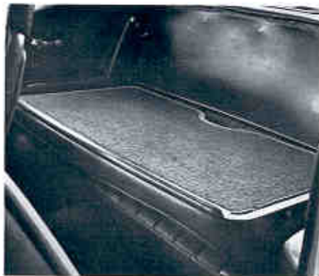
Fold-down Rear Seat (Code 604—UPC A67). Firebird only. Nylon-blend, deep-loop carpeted rear seatback. Folds down neatly to accommodate bulky objects. Carpeting matches interior. (F)
