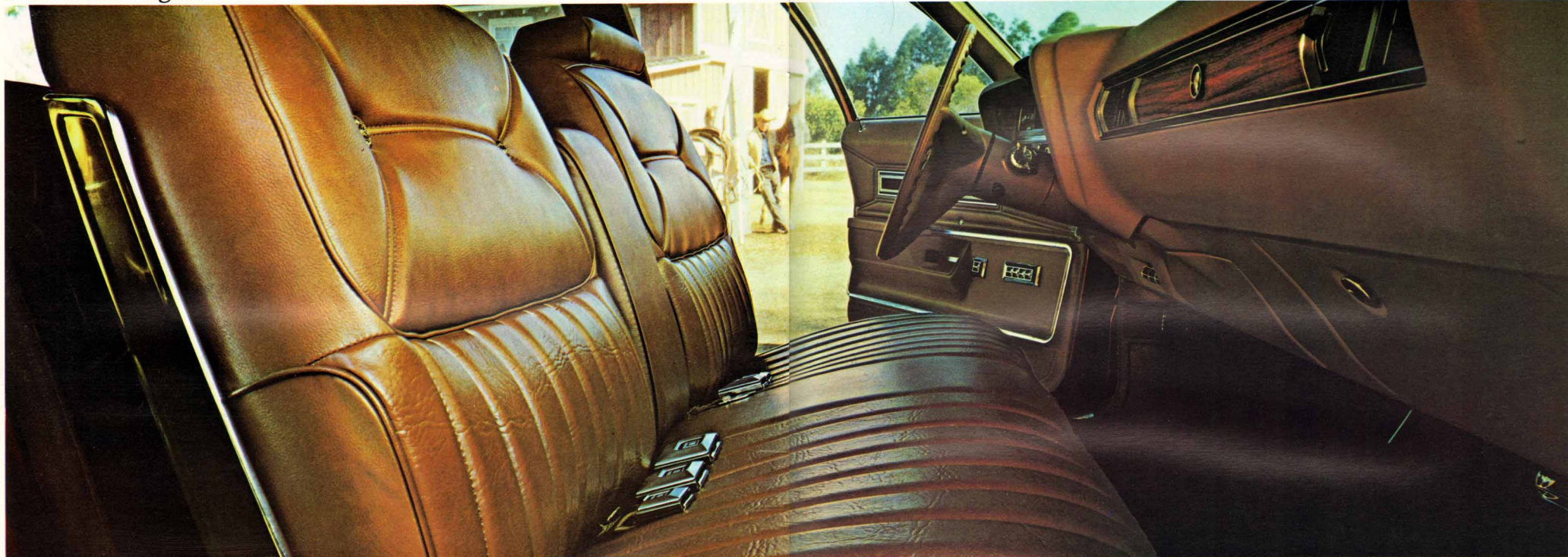
Elk-grain expanded vinyl and Madrid-grain vinyl notchback seat shown in Saddle (1).
