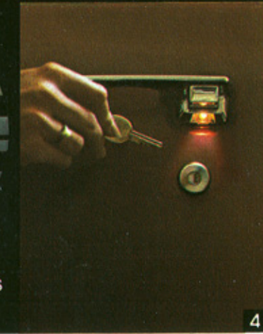
2 This Landau vinyl roof may be ordered. An elegant touch. 3 Controls are lighted by tiny flood lamps. 4 Door lock button lights the exterior lock and car's interior, available. Turns off automatically in about 30 seconds. 5 60/40 seat, available. 6 Standard Luxury Sedan Armrest Bench seat. 7 Ninety-Eight Luxury Sedan.
