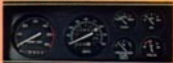
Available instrumentation — with voltmeter, temperature and oil pressure gauges, plus trip odometer. Standard on Calais.
