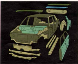
Extensive anti-corrosion measures. Includes galvanized metals, front fender liners, plastisols, sealers, waxes and zinc-rich primers. All to help keep Omega looking good.
