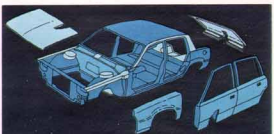
Extensive anti-corrosion measures. Includes galvanneal metals, plastisols, sealers, front fender liners, waxes and zinc-rich primers.
