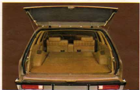
Split-tailgate. Top swings up. Bottom drops down for a loading platform on Cruiser.
