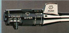
Cruise Control with "Accel" feature. Lets you accelerate to desired speed and hold it. Any-one who's ever taken a long trip wouldn't be without it. Standard on Toronado.
