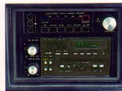
Delco AM-FM stereo with graphic equalizer, cassette, clock, Electronic Touch Climate Control
