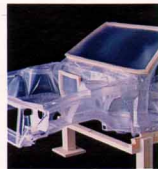
Plastic scale models—this is the front of the new Electra—are used to evaluate designs. Some are even barrier tested.
