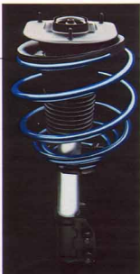
Space-saving MacPherson struts and concentric coil springs are used in the Electra's front suspension.
