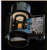
The mass air-flow sensor provides an on-board computer with information critical to maintaining proper air-fuel mixture.
