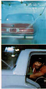
In the check for water leaks, a pressurized water and dye mixture is sprayed on at a simulated 40 mph. A "black light" instrument, which makes the dye visible, indicates any leaks.
