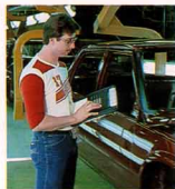
The Data-Mite hand-held computer is also used in the visual inspection of the finished paint job.
