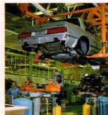
An engine and chassis are "married."
