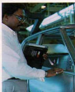
Using a hand-held computer called a Data-Mile, an inspector makes a record of his detailed quality checks on the assembly line.
