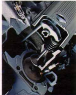
With sequential-port fuel injection, fuel is metered directly into each combustion chamber.
