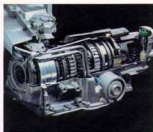
A new four-speed automatic transmission with overdrive is computer-controlled.
