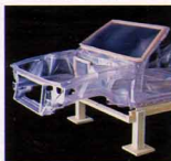
Structural scale modeling has led to lighter, stronger Buicks.
