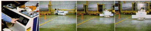
A driverless "Towveyor" follows an electrical cable buried in the floor to efficiently deliver parts to work stations throughout the assembly area.
