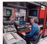
Test engines are run hundreds of hours wide-open on the dynamometer.
