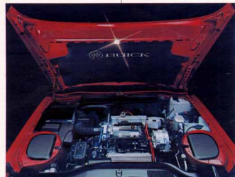
Electra's transverse engine arrangement allows better passenger accommodation in a smaller package.
