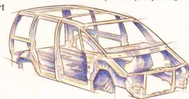
Silhouette uses a space-frame steel structure to help protect you and your passengers.
