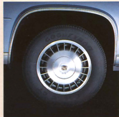
15" Aluminum Alloy Wheel and Goodyear Eagle GT Tire.
