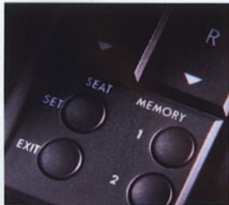
A DRIVER'S-SEAT MEMORY RECALLS TWO PREFERRED SEATING POSITIONS AND A PROGRAMMABLE EXIT SETTING.
