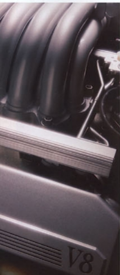
TUNED AIR INTAKE RUNNERS IN THE HIGH-OUTPUT V8 PACK AIR MORE DENSELY IN THE CYLINDER TO PRODUCE GREATER POWER.
