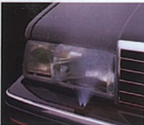
A WASHER HELPS KEEP ALLANTÉ'S INTEGRATED HEADLAMP/FOGLAMP CLEAN FOR MAXIMUM VISIBILITY.
