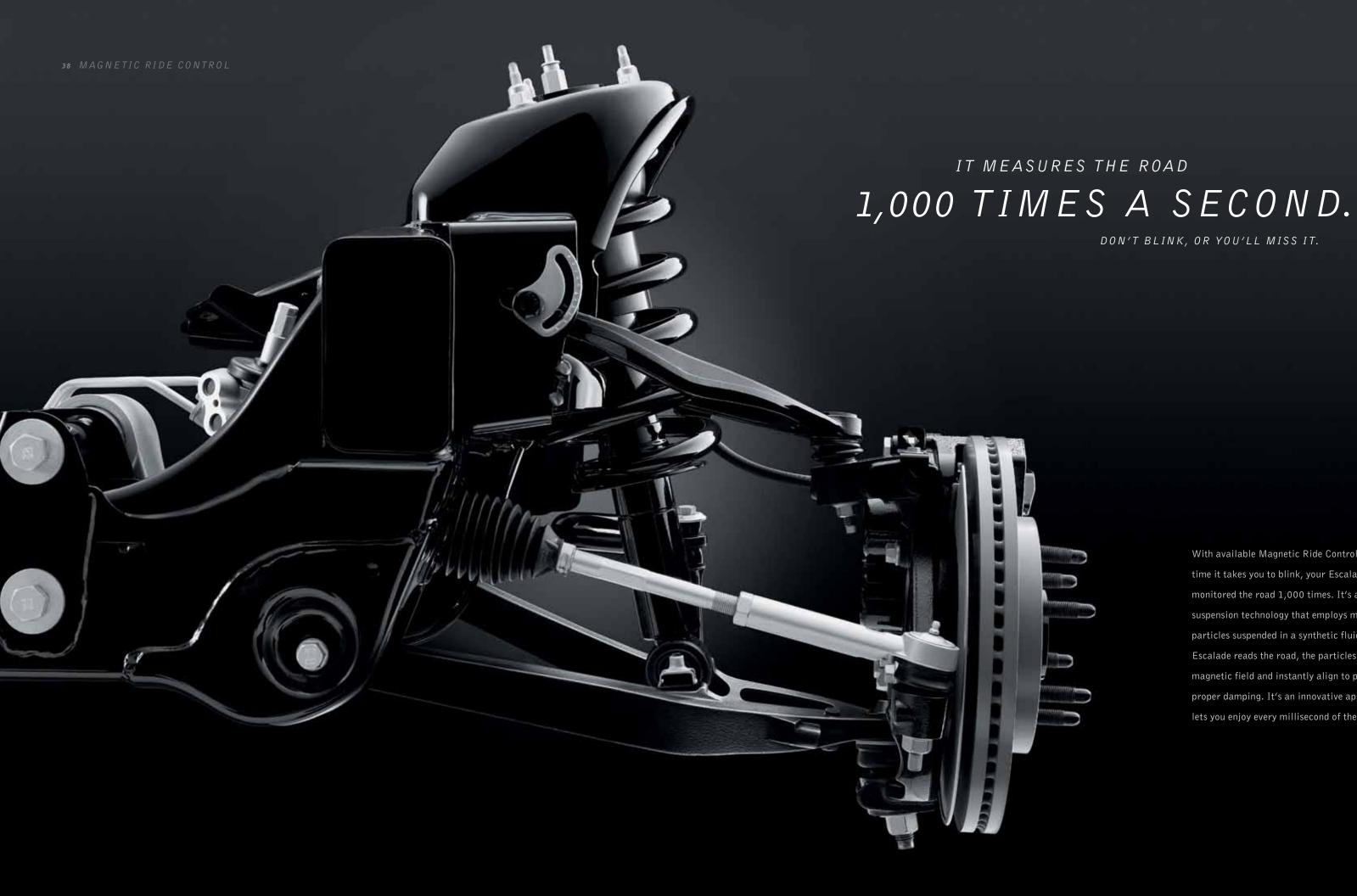
With available Magnetic Ride Control, in the time it takes you to blink, your Escalade has monitored the road 1,000 times. It's an ingenious suspension technology that employs minute iron particles suspended in a synthetic fluid. As the Escalade reads the road, the particles react to a magnetic field and instantly align to provide the proper damping. It's an innovative approach that lets you enjoy every millisecond of the ride.
