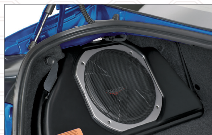
10-inch Powered Subwoofer. Provides powerful, deep bass and also assists in clean sound reproduction from all vehicle speakers. This is achieved by its integrated 100W amplifier and a passive crossover network. The self-contained unit mounts in the trunk. Manufactured for Subaru of America by Kicker®. Cannot be installed with Cargo Tray.
