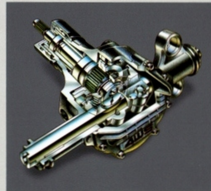
Unique, all-mechanical rear wheel steering box.
