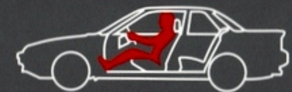
Ergonomic, cockpit-like interior with 43.1 in. legroom and 36.9 in. headroom.
