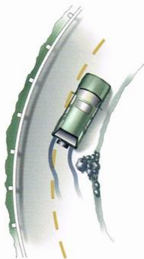
The 4-Wheel Anti-Lock Braking System on the Passport 4WD EX model can help the driver retain steering control during heavy braking.
