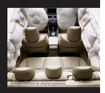
Every Accord comes standard with dual-stage, multiple-threshold front, dual-chamber front side and side curtain airbags to help reduce the likelihood of injuries in a collision. The front passenger's side airbag uses the Occupant Position Detection System (OPDS) to prevent deployment if a child or small-statured passenger is out of position and in the airbag's path of deployment.
