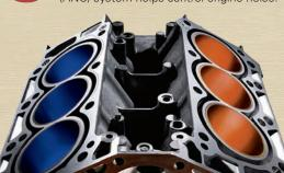
When maximum torque is required—such as when you're merging onto the freeway or climbing a steep hill—all six cylinders are firing to deliver the engine's full power.
