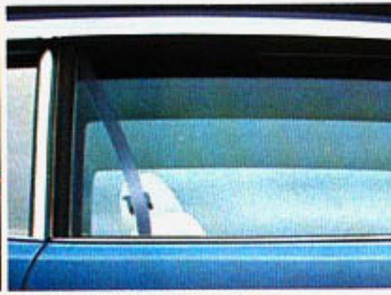
Power windows. Raise or lower windows at a touch of a button.
