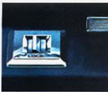
Power door lock system. Controls on each door allow driver or passenger to lock or unlock both doors instantly.
