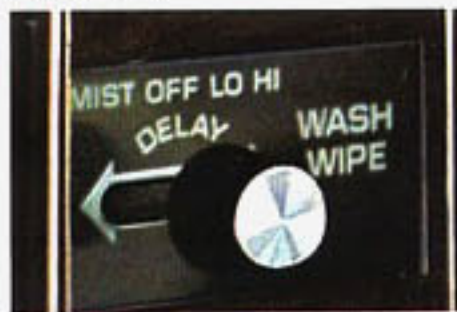
Intermittent windshield wiper system. Varies the wipe cycle from 1:2 to 20 seconds to adjust for light drizzle or mist.
