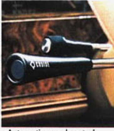
Automatic speed control. Automatically maintains a constant speed for added driving ease during long stretches.
