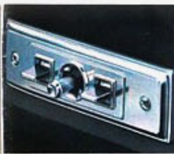
Power seat. Electric 6-way control of entire front seat, or driver's seat only if ordered with 55:45 seats.
