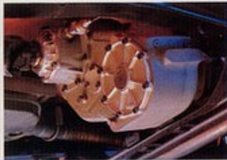
New lightweight aluminum transfer case with synchronized gears enables you to shift from 2WD to 4WD at speeds less than 20 MPH.
