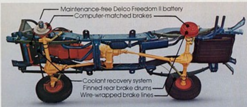
Blazer chassis has drop-center frame design for a low silhouette and easy entry height. It's loaded with rugged truck features.
