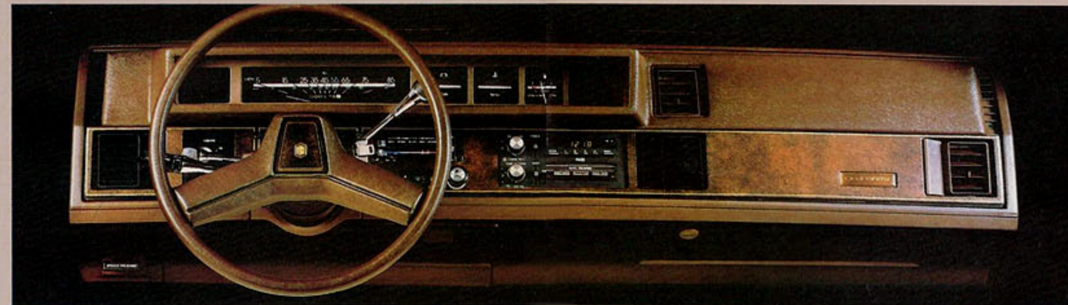
Celebrity CL instrument panel. Note: Speedometers in Canada have major scale in km/h, secondary scale in MPH and odometer in kilometres.
