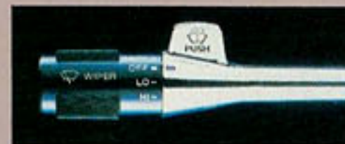
Column-mounted multi-function lever controls for windshield washer and wipers, hi/lo beam and turn signal.
