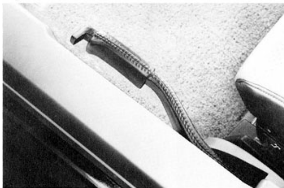
Left-Hand Operated Parking Brake Returns to Downward Position after Application
