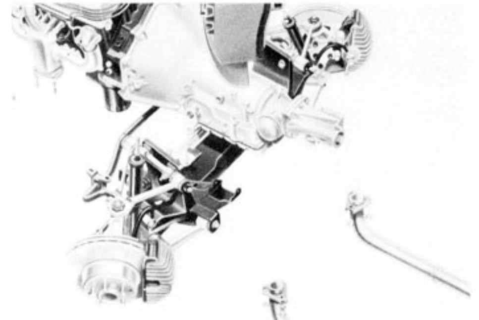
Forged Aluminum Upper and Lower Control Arms and Spindles
