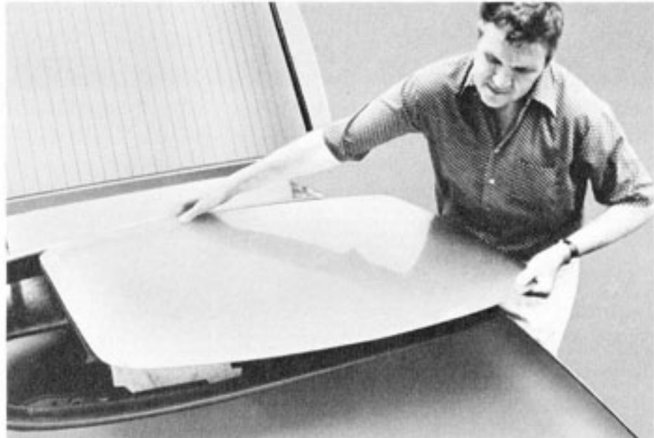
One-Piece Lift-off Roof Panel; Eliminates the T-bar Configuration
