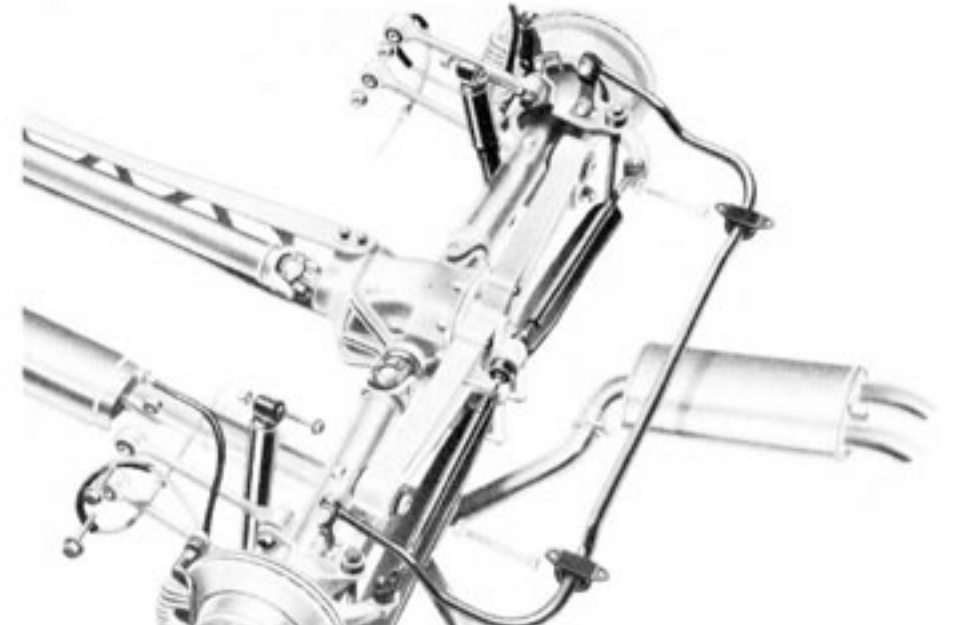
Five-Link Rear Suspension with Transverse Glass-Epoxy Composite Spring
