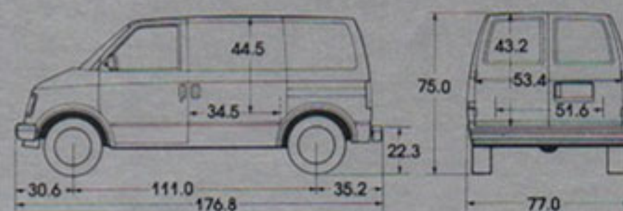
Dimensions (in inches) shown are with standard equipment and the vehicle is unloaded.
