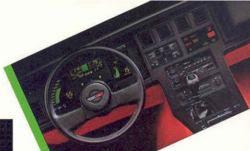
■ Corvette's electronic instrument cluster includes both graphic and numeric displays for instant communication.
